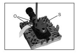
Loosen the clamping brackets (S) on the valve heads (O).
