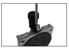
Loosen connection fastener slightly.
