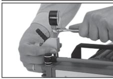
Assemble control valve first, then align and fasten gauge.
