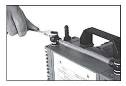
Use open-ended wrench, remove screw-in fittings from all pump heads.
