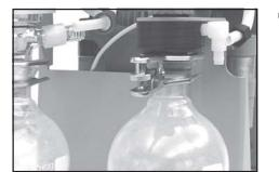
Remove union nut at the exhaust waste vapour condenser and remove hose from the inlet of the condenser.
