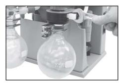
Tighten union nut first by hand and then tighten by one full turn using open-ended wrench.
