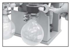
Use open-ended wrench (w/f 17) to remove union nut on the fitting of the cover plate.
