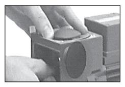
By turning eccentric bushing (front of connecting rod), bring connecting rod into a position in which diaphragm is in contact with housing and centred with respect to bore.
