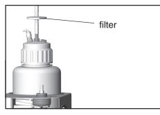
Ensure that there is no liquid in the tube, risk of contamination! Remove connecting tube from the filter. Remove the filter from the piece of tube at the hose nozzle. Assemble new filter (position with the printed side towards the bottle) and assemble connecting tube.
