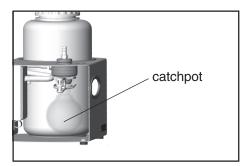
The hydrophobic filter retains water and aqueous solutions also in the form of aerosols. When using solvents or due to evaporation of water, condensate may be recovered in the catchpot. Remove joint clip and catchpot and drain condensate in case.
