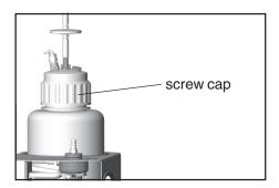
Check level of liquid in the collecting bottle regularly. **Maximum liquid level in collecting bottle:** approx. 80 %, depending on the application (in case of low boiling liquids or in case of suction of liquids which tend to foam, the maximum liquid level might be reduced).
