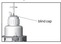
Remove the blind cap. Remove screw cap from bottle. Insert lead-through (2) with coupling (1) (Attention: Parts are sealed with adhesive for leak tightness) and with seal ring (3) to screw cap and assemble hose (5) under the screw cap with locknut (4). Adjust hose towards flask wall. Assemble screw cap.
