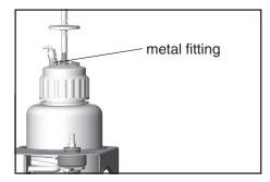
Do not remove the **metal fitting** at the screw cap. If the fitting is loose, tighten the fitting carefully.
