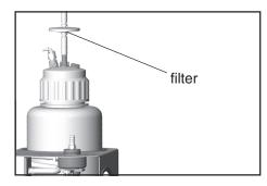
Change filter if necessary (contaminated, no or bad aspiration, pressure control device switches without demand of vacuum).
