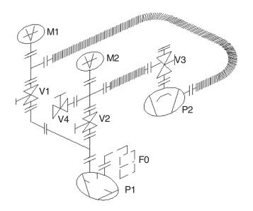
P1 backing pump P2 diffusion pump V1 foreline valve V2 by-pass valve V3 high vacuum valve V4 venting valve M1 measuring point 1 M2 measuring point 2 F0 oil mist filter
