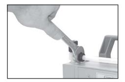
Tighten union nuts first by hand and then tighten one full turn using open ended wrench (w/f 17).
