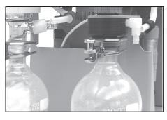
➡ Remove union nut at the exhaust waste vapour condenser and remove hose from the inlet of the condenser.
