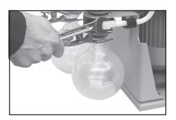
Use open-ended wrench to reconnect hose to elbow fitting.
