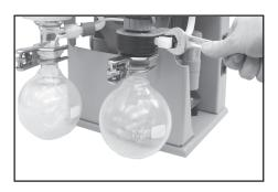
➡ Tighten union nut first by hand and then tighten by one full turn using open-ended wrench.
