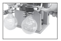
➤ Use open-ended wrench (w/f 17) to remove union nut on the fitting of the cover plate.
