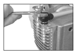
→ Use an open end wrench (width 17) to assemble the screw-in fittings with connection hose to the pump heads. In case, steady with an open end wrench (width 20).
