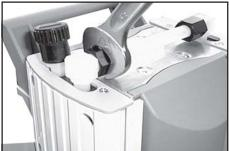
Use open-ended wrench to remove union nut at hose connection next to the gas ballast.
