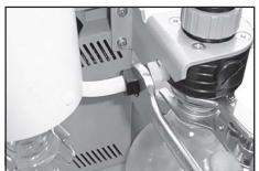
Connect hose to fitting. Tighten union nuts first by hand and then tighten one full turn using open ended wrench.
