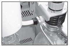
Use open-ended wrench to remove union nut at the inlet of the pump. Remove hose from the fitting. Do not remove the elbow fitting from the pump head. Through reassembly a leak may result.
