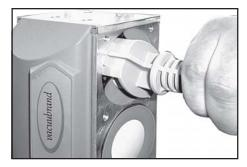
Make sure that the square head screw of the diaphragm clamping disc is correctly seated in the guide hole of the diaphragm support disc.
