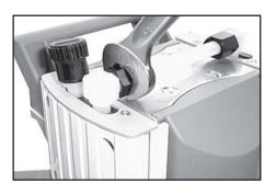
Use open ended wrench to reconnect hose to elbow fitting. Tighten union nuts first by hand and then tighten one full turn using open ended wrench.
