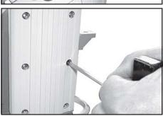
Use hex key to remove six socket head screws from pump head and remove upper housing (housing cover, housing cover insert and head cover).
