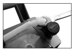
Slip the hose onto the hose connector by turning the fitting (L) with an open-ended wrench w/f 14
