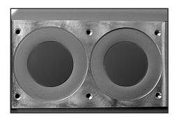
Check diaphragms (E) for damage and replace if necessary.
