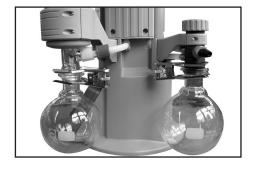
→ Assemble catchpots (10) with joint clips.
