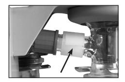
Replacing the overpressure safety relief device:
