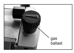
For **condensable vapors** (water vapor, solvents, etc.):
