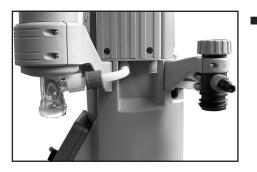
Remove catchpots (10) at inlet and outlet (see "Use and operation", page 38).
