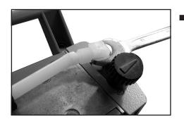
Slip the hose onto the hose connector by turning the fitting (L) with an open-ended wrench w/f 14.
