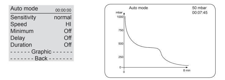
When selecting "Graphic" the display shows a pressure vs. time curve.
