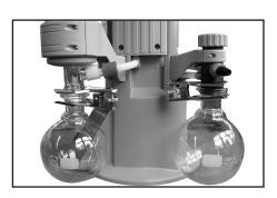
➡ Assemble catchpots (10) with joint clips.
