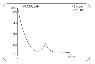
When selecting "Graphic" the display shows a pressure vs. time curve.
