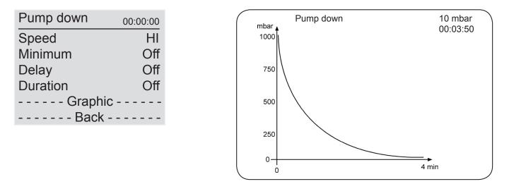
When selecting "Graphic" the display shows a pressure vs. time curve.
