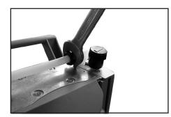
Loosen the union nut (K) of the hose connection next to the gas ballast valve with an open-ended wrench (w/f 17).
