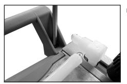
Attach the handle at the housing cover (use 5 mm wide Allen key)
