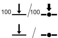
Vacuum control to a preset vacuum value (here: 100 mbar/Torr/hPa); (without / with VACUU•BUS-compatible VARIO pump)
