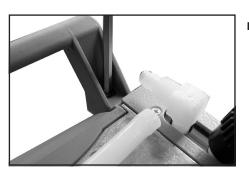
Loosen the screw affixing the handle (use 5 mm wide Allen key) at one housing cover.
