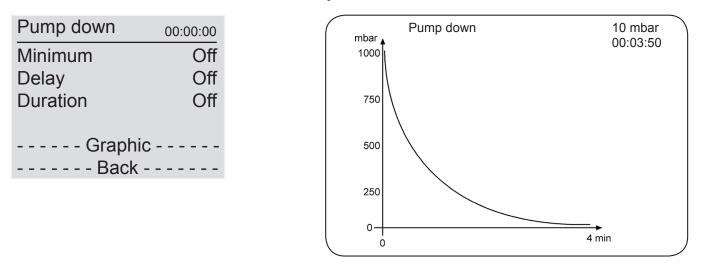
When selecting "Graphic" the display shows a pressure vs. time curve.
