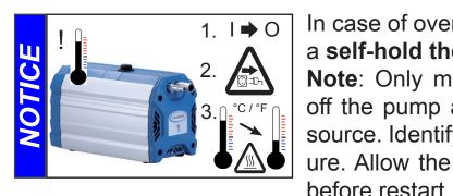
In case of overload, the motor is shut down by a **self-hold thermal cutout** in the winding. **Note**: Only manual reset is possible. Switch off the pump and disconnect from the power source. Identify and eliminate the cause of failure. Allow the pump to cool down sufficiently
