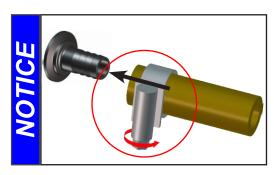
Secure hose connections at the pump appropriately, e.g., with hose clamps, to protect against accidental detachment.
