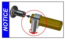
Secure hose connections at the pump appropriately, e.g., with hose clamps, to protect against accidental detachment.
