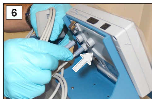
6. Also plug in the VACUU·BUS cables from peripheral devices. Use Y adapters (accessories) if there are not enough connections.
