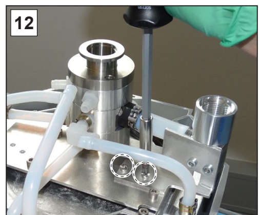
12. Wind in the screws at the outlet holder hand-tight; Phillips screwdriver size 2.
