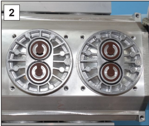
2. Insert the new O-rings into the grooves. Insert the new valves. Pay attention to the correct orientation of the valves.
