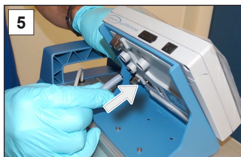
5. Plug the VACUU·BUS cable into the power connection on the back of the controller.
