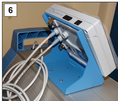
6. Secure the controller on the diaphragm pump and connect all cables.
