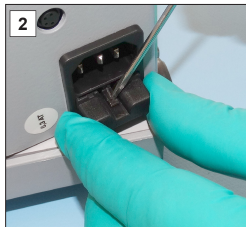
2. Carefully pull out the fuse holder.
